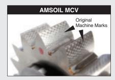
Pass Example: Passed Stage 13, Total Wear, **0mm**
