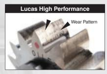
**Failure Example:** Passed Stage 11, Failed Stage 12, Total Wear in Stage 12, **160mm**
